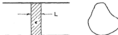
Fig. 1—Transverse dielectric slab window.
